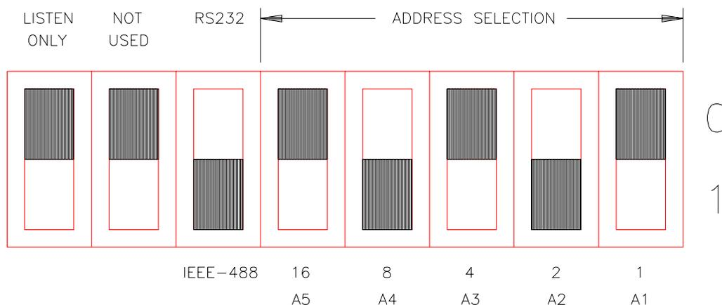
**Figure 13-1: GPIB Address Selection Switch**
