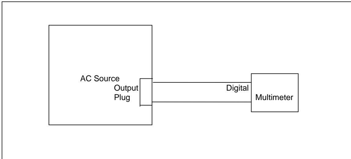
**Figure 6-1: Test Equipment Hookup for Routine Output Calibration**
